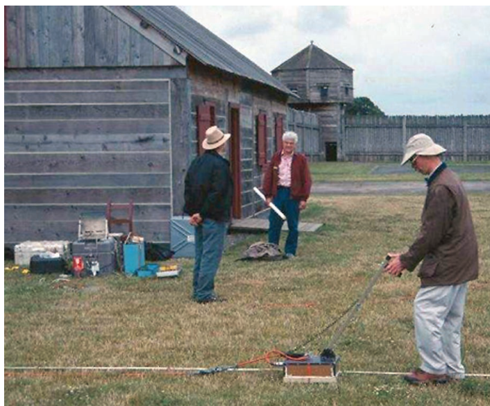
Figure 2. Ground Penetrating Radar (GPR) looks like a “lawn mower” and detects underground disturbances (Feder 2004: 91).
